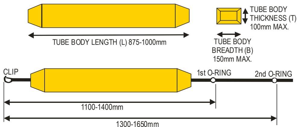
The distance from the extremity of the clip to the extremity of the first O-ring shall be a minimum of 1.10 m to a maximum of 1.40 m.
